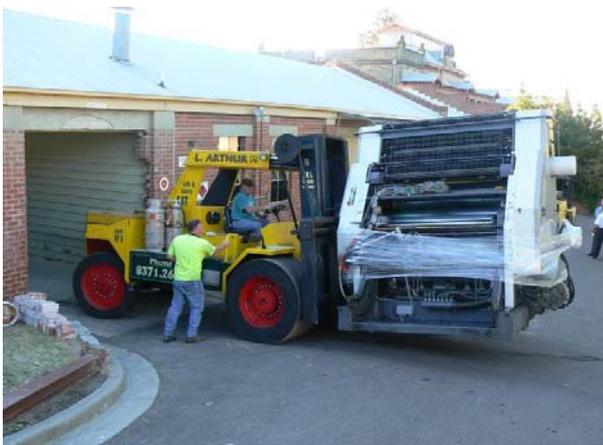
The photo at left shows the 50 tonne forklift moving the first of the two Roland decks out of the Litho Despatch door. Note the bricks missing where the doorway had to be enlarged after the rolla-door was removed to allow some larger pieces egress. The heaviest piece of equipment is said to have weighed approximately 30 tonne.
